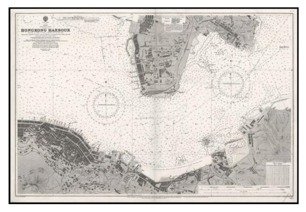
Engraved chart, inset conversion table of feet to meters, shows details of land being reclaimed.
