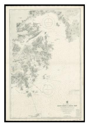
Engraved chart, including tidal information, compass roses, soundings, seabed notations, currents, sandbanks, shoals, lighthouses and beacons picked out in yellow and red, inland elevations, detailing, and buildings, paste-over showing dredged area in red, and plotting of a ships tack.
