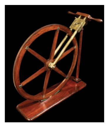
Signed to dial Dixey & Sons, London, with engraved brass dial divided for furlongs, miles, poles and yards, six-spoke wheel with steel rim tread, square brass fork body with hinged side for wheel removal, straight handle, on modern mahogany stand.
