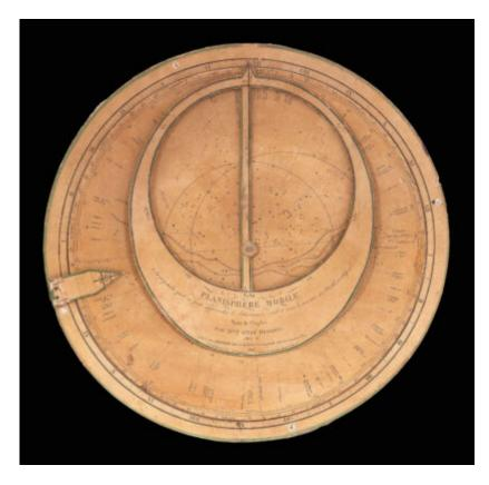
Revolving planisphere, essentially a large volvelle, four moveable discs of engraved paper over pastboard, edges painted green, held together by a brass screw, paste-board pointer. A little toned.
