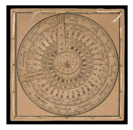
Engraved astronomical instrument on card with internal rotating disc and two pointers in verso.
