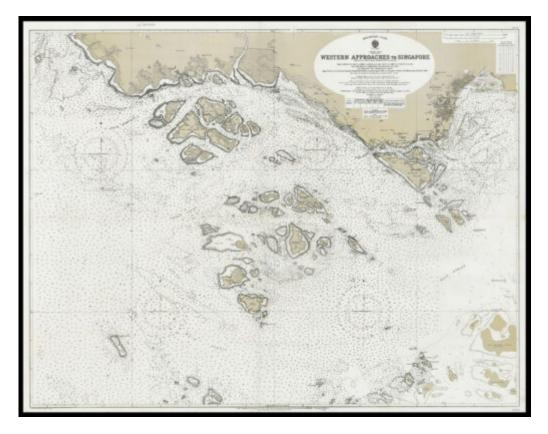
Engraved chart, including tidal information, compass roses, soundings, seabed notations, sandbanks, shoals, lighthouses and beacons picked out in yellow and red, inland elevations and detailing, a few red ink arches showing the radius of lighthouse illumination, inset chart of Tai Sami, and Goat Island.
