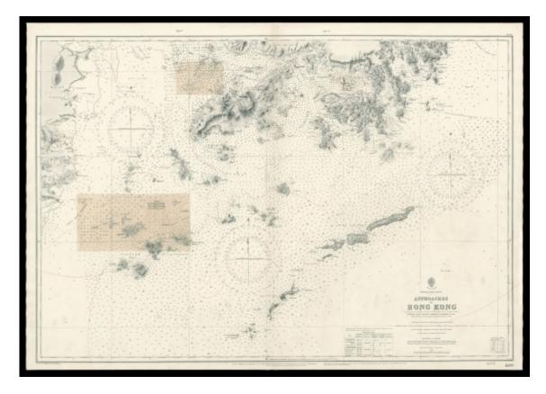
Engraved chart, including tidal information, compass roses, soundings, seabed notations, currents, sandbanks, shoals, lighthouses and beacons picked out in yellow and red, inland elevations and detailing, with two paste overs.
