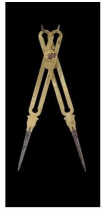
Six-inch proportional dividers, brass body, steel point, with engraved units on both sides.
