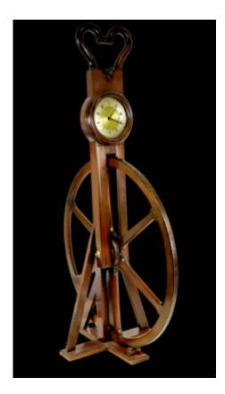
Signed to dial Dollond, London, with engraved brass dial divided for Furlongs, Miles, Poles and Yards, six-spoke wheel with steel rim tread, square mahogany fork body with hinged side for wheel removal, hoop handle, on modern brass and mahogany stand.
